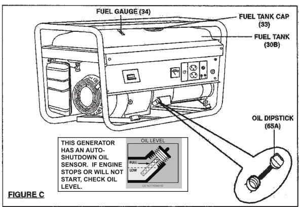
3. Before the first use, remove the Fuel Tank Cap (33B<sub>1</sub>) and fill the Fuel Tank (30B<sub>1</sub>) with **unleaded** gasoline. Then, replace the Fuel Tank Cap. If necessary, refill the Fuel Tank with unleaded gasoline. (See Figure C.)
